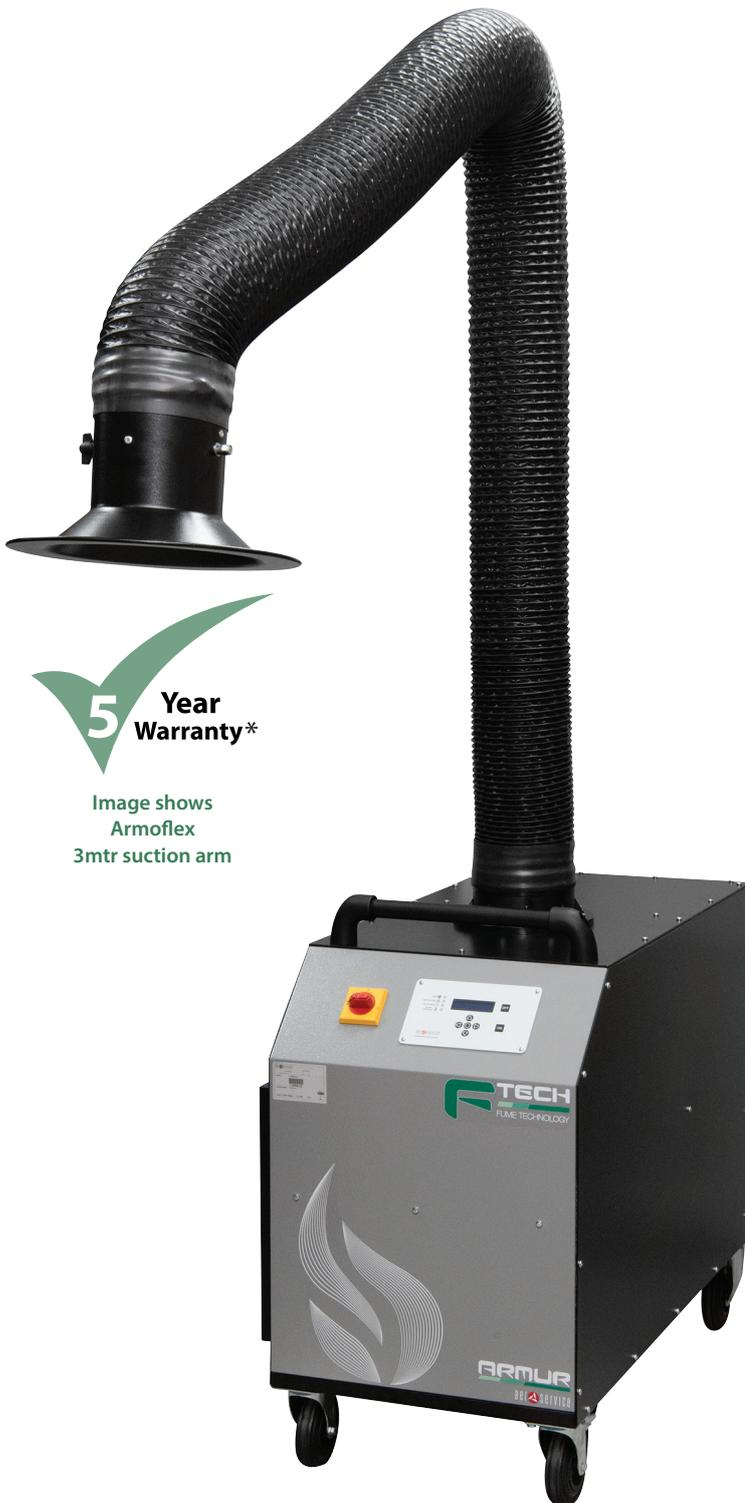
The F-Tech Armur is a high performance mobile extraction system designed for extraction and filtration of fumes derived from the welding processes, micro dust, vapours and odours.
